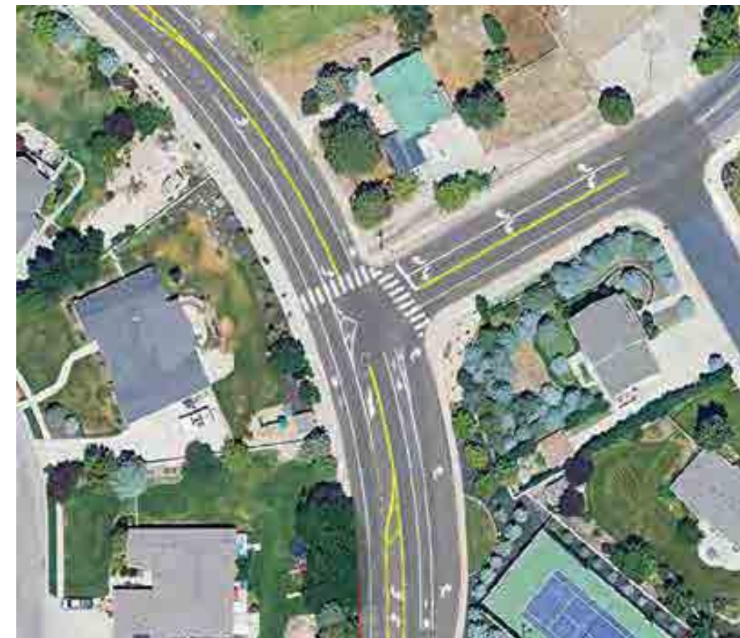
Proposed high-T design at Canyon Crest Road and Ridge Drive with left-turn merge lane and restriping
