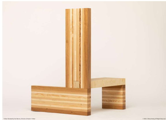
B.2.4: GLU-LAM TIMBER POST AND BEAM
