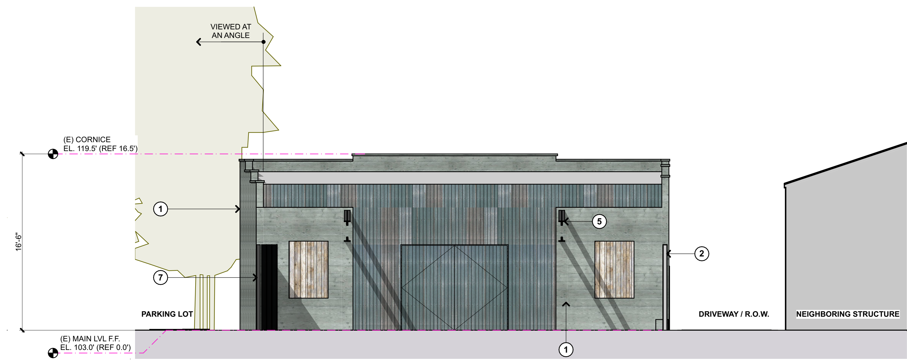
4 EAST ELEVATION - EXISTING SCALE: 3/16" = 1'-0"
