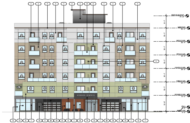
2 SOUTH ELEVATION Facing Seymour Street 3/32" = 1'-0"
