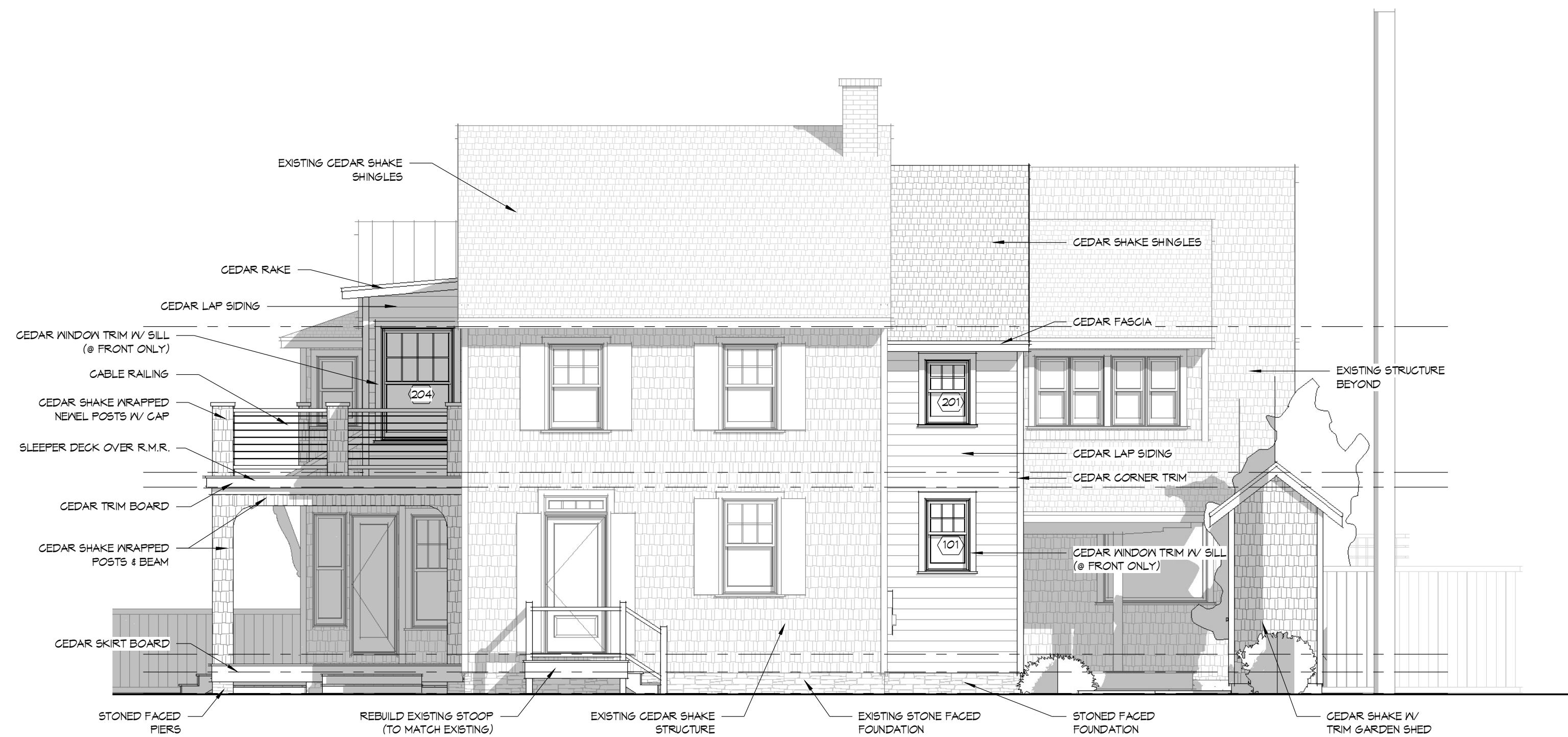
① RIGHT SIDE ELEVATION (PROPOSED) 1/4" = 1'-0"
