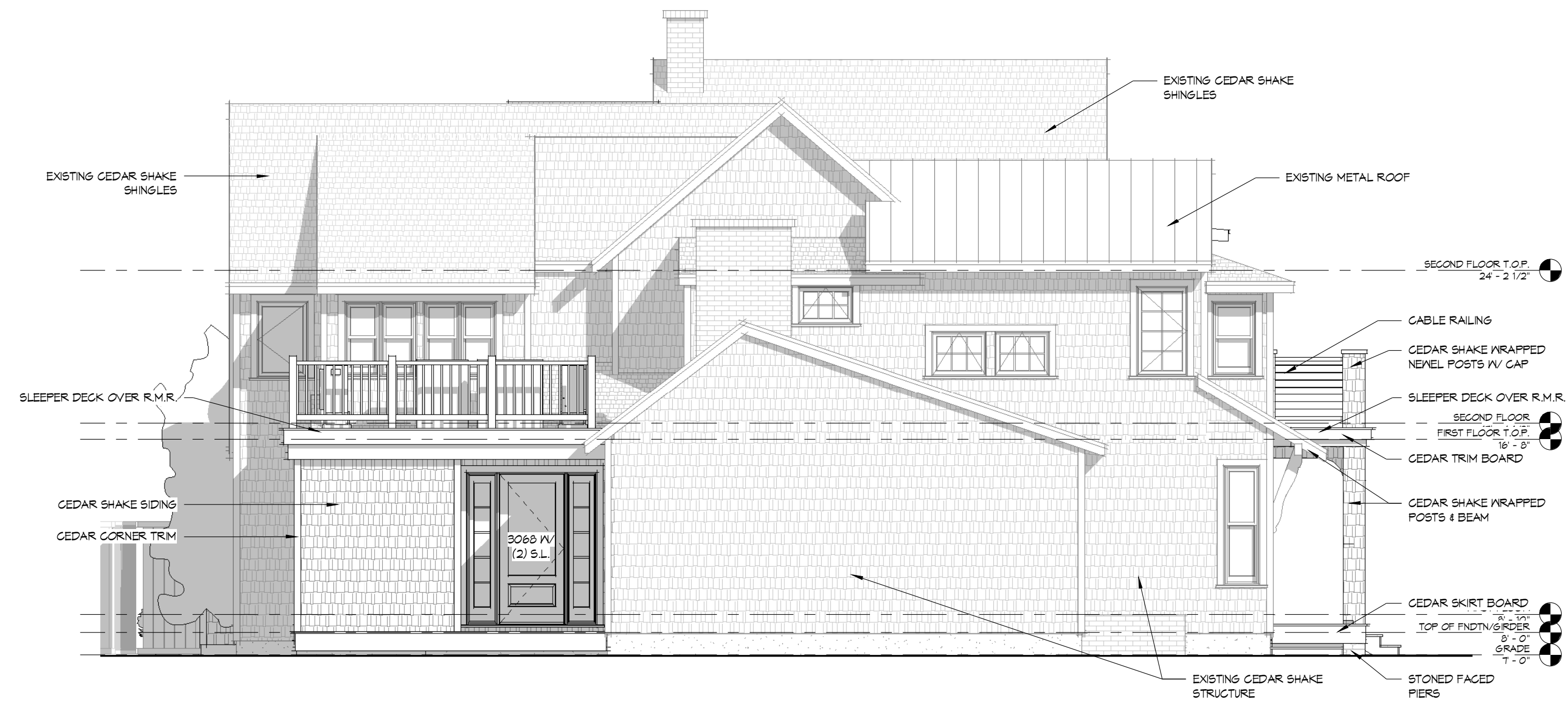
② LEFT SIDE ELEVATION (PROPOSED) 1/4" = 1'-0"
