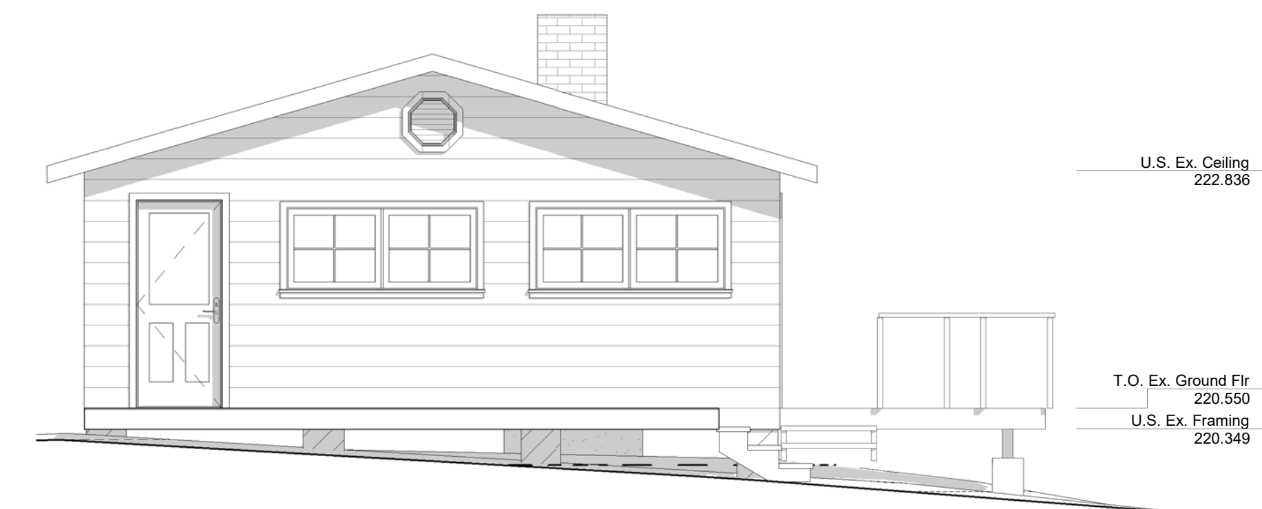
1 Existing North Elevation 1 : 50
