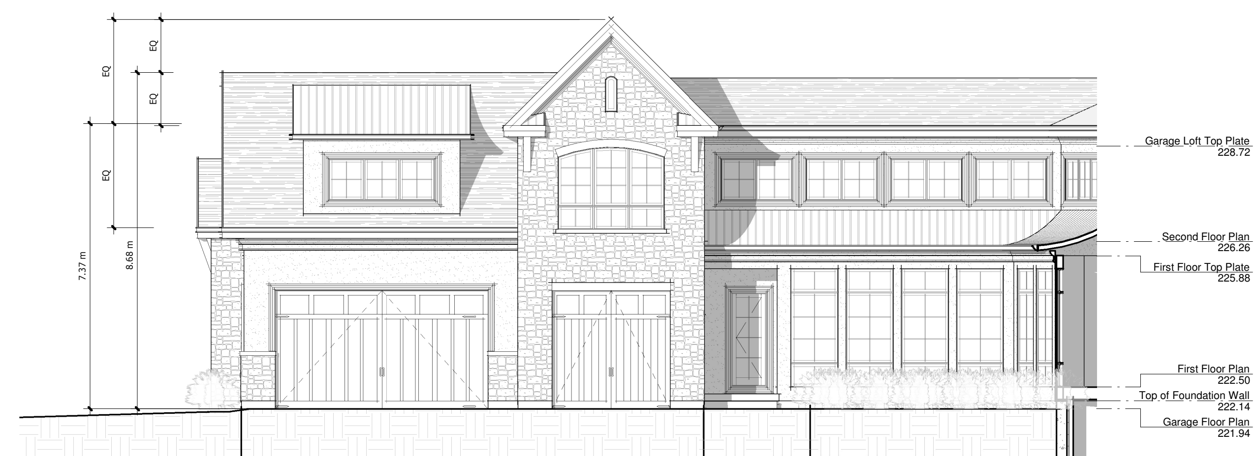
South Elevation - Garage 1/8" = 1'-0"
