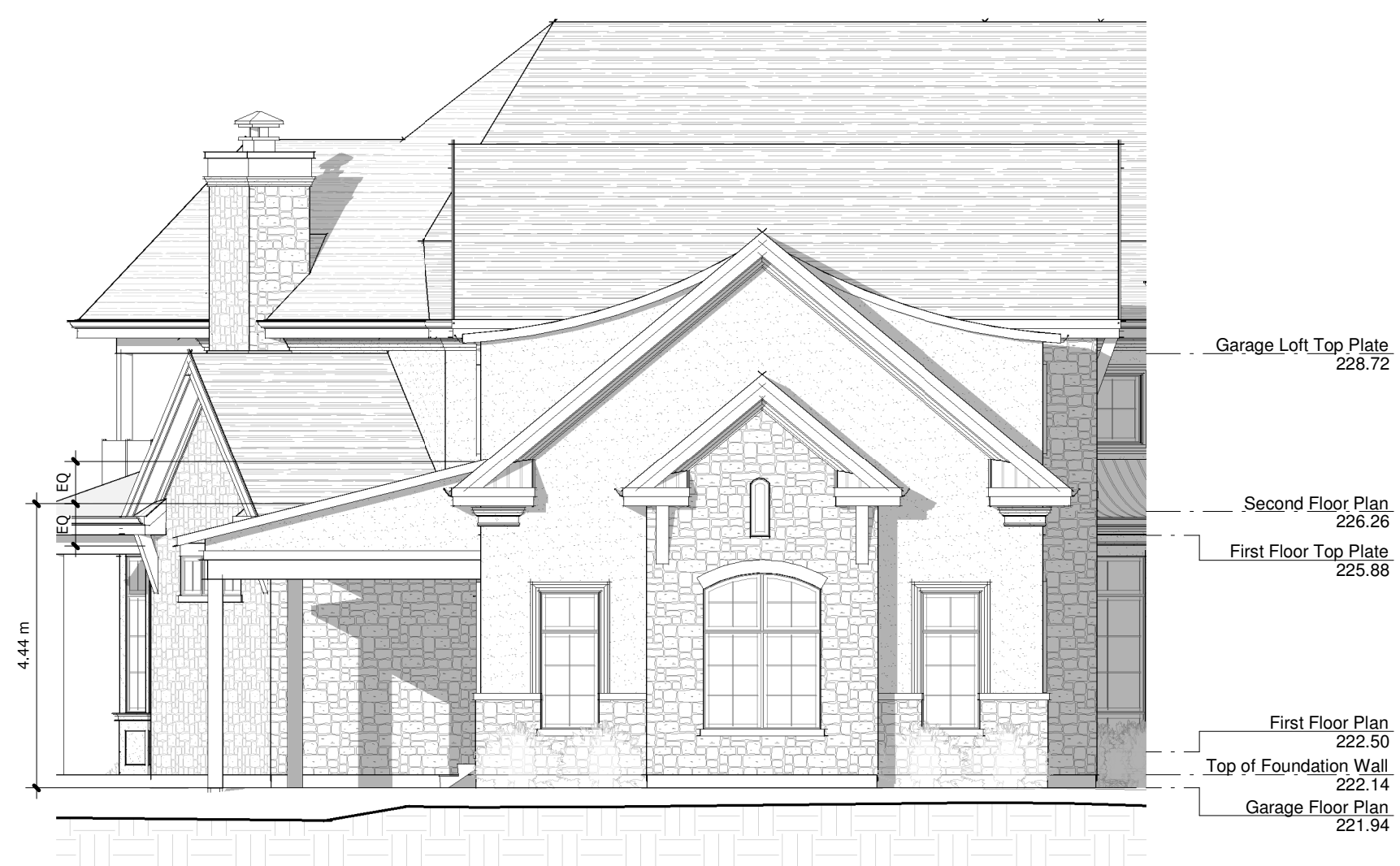
West Elevation - Garage 1/8" = 1'-0"
